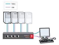
The switching section is hard wired to allow only one channel to be selected at any time. Common keyboard, mouse and video monitor are able to access multiple monitor are able to access multiple high security computers/networks, safe in the knowledge that data will not be transferred from one to another, either by user error or subversive attack.
